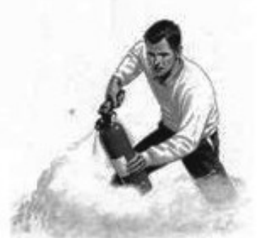
S weep the source of the flames until the extinguisher runs dry
